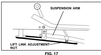
FRONT-TO-BACK ADJUSTMENT (See Figs. 18 and 19) IMPORTANT: DECK MUST BE LEVEL SIDE-TO-SIDE. IF THE FOLLOWING FRONT-TO-BACK ADJUSTMENT IS NECESSARY, BE SURE TO ADJUST BOTH FRONT LINKS EQUALLY SO MOWER WILL STAY LEVEL SIDE-TO-SIDE.
